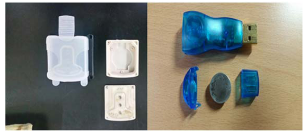
Fig. 6. PPSF case covered with heat resistant silicone cover(left) and button type temperature logger (right).
